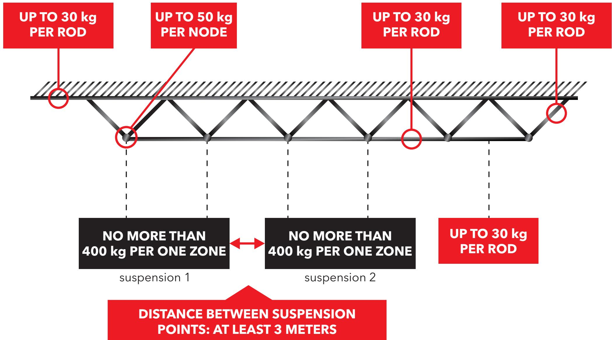
\*In the winter period, the total weight of the suspended structure must be reduced by 30%.
