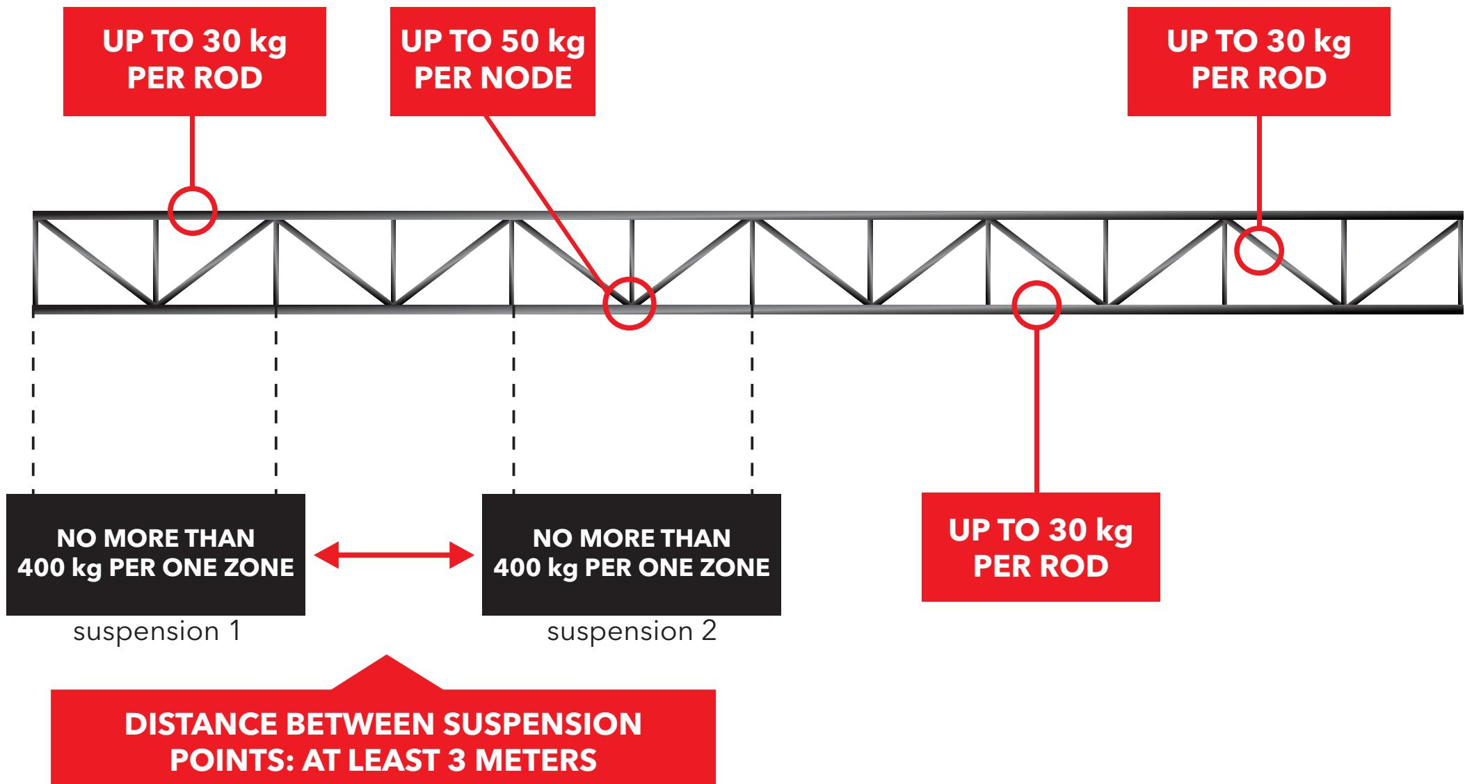
\*In the winter period, the total weight of the suspended structure must be reduced by 30%.
