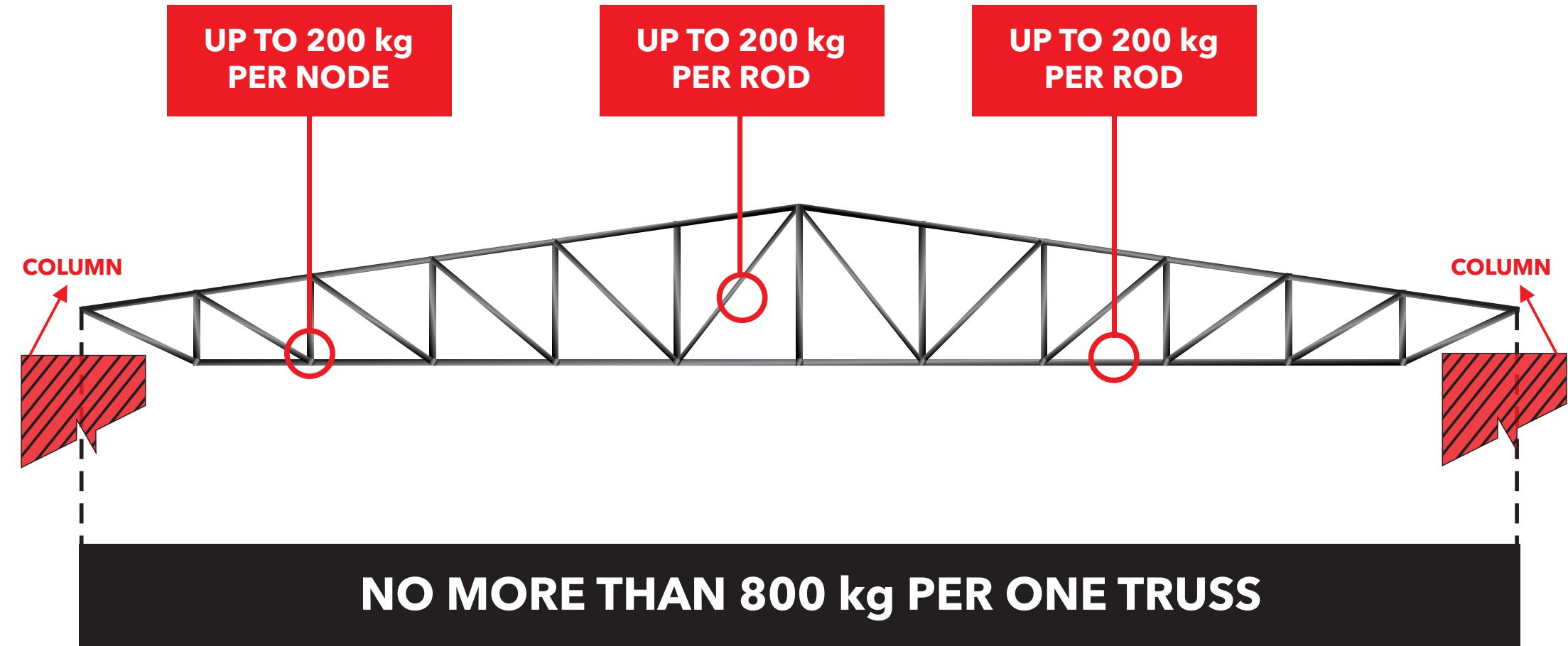
\*In the winter period, the total weight of the suspended structure must be reduced by 30%.
